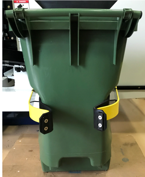
65-Gallon Can with Belt Bolted Through Middle Set of Holes on Belt and Bracket
