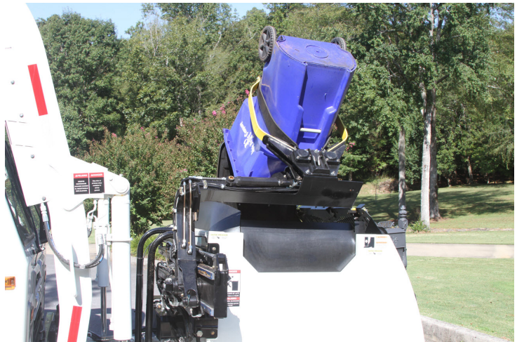
Fig. 3-13 Showing Lift Function Alone
