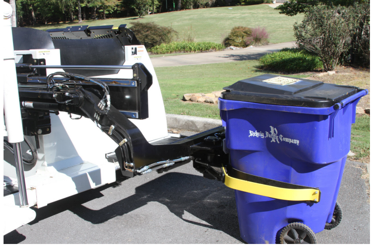
Fig. 3-12 Maximum Arm Extension is 60"
